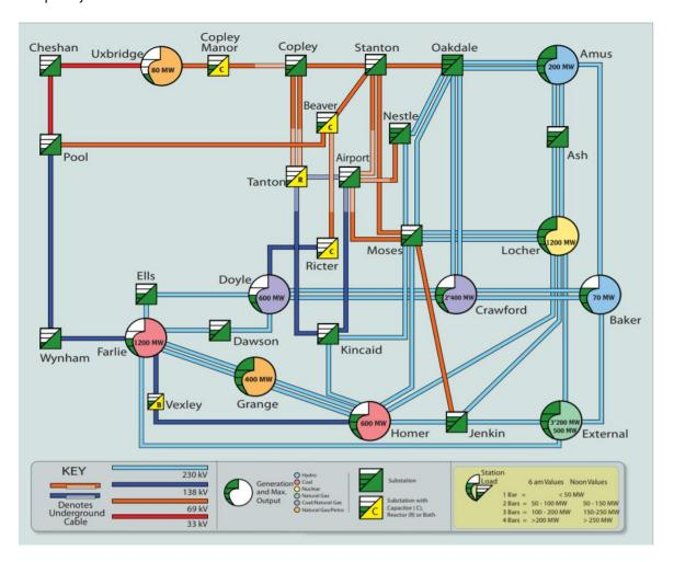
The PALCO system is complex enough so that students can experience all the types of operating problems that occur on actual systems. The model includes details on a variety of substation breaker configurations including double breaker, breaker and half, and single bus-single breaker configurations.
